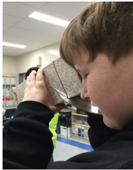
Left: Checking out the spectrum of light emitted by the ceiling light using the spectroscope we made with CD and cardboard box.
